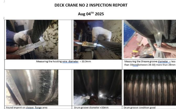
Figure 1. Diameter incompatibility between the hoisting wire rope and the groove dimensions of the drum and sheave observed MV Roslyn .
